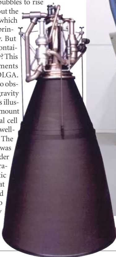
Vinci engine under development. This liquid hydrogen - liquid oxygen engine completed its preliminary reignition tests at the Lampoldshausen rocket engine test facility (Germany) in 2007. Inset: the complete engine with its divergent nozzle.
