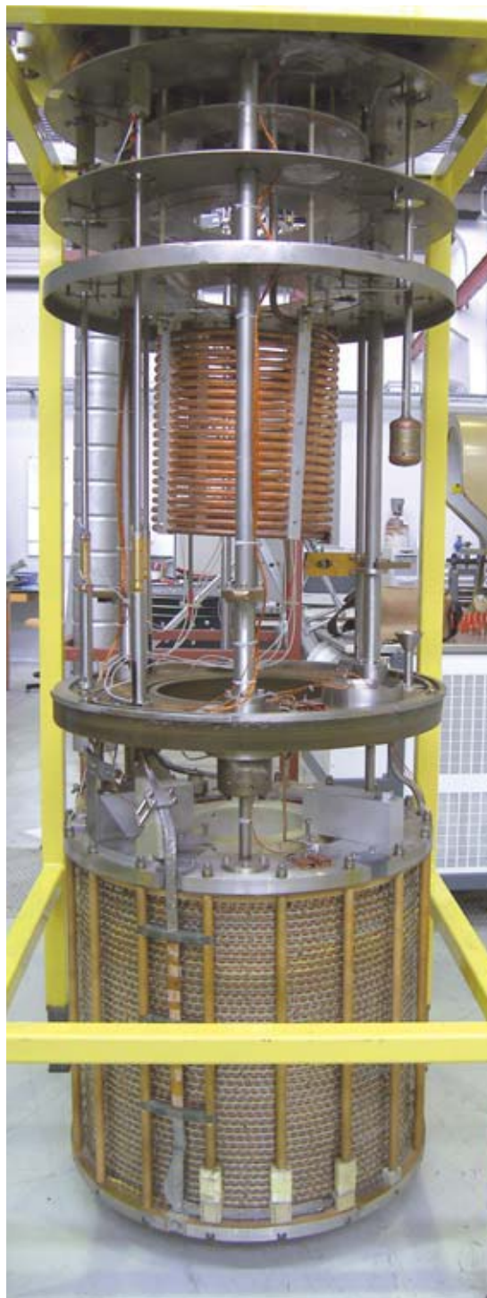
The superconducting coil at the OLGA facility, at the CEA centre in Grenoble.
